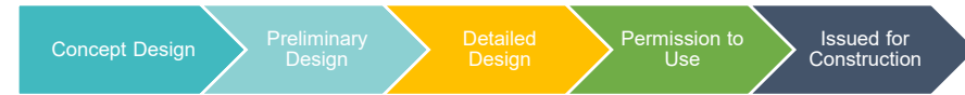
Figure 6 Each ESC plan and drawings is subject to a four-gate design review process for each progressive stage of construction
