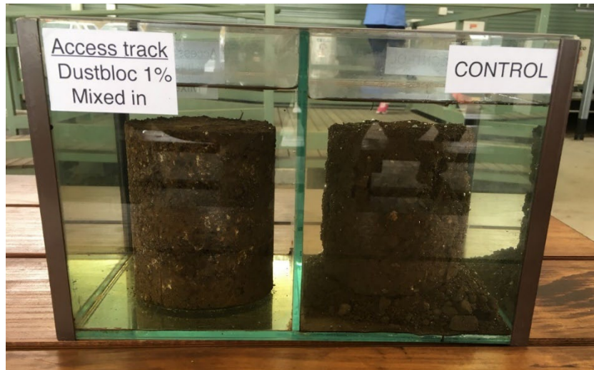
Figure 16 A trial using Dustbloc demonstrated the effectiveness of this simple solution.
