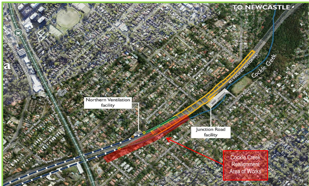
Figure 3: Close up of the northern civils package at Wahroonga, highlighting Cockle Creek along the southbound alignment of the M1 Pacific Motorway, and the realignment work area
