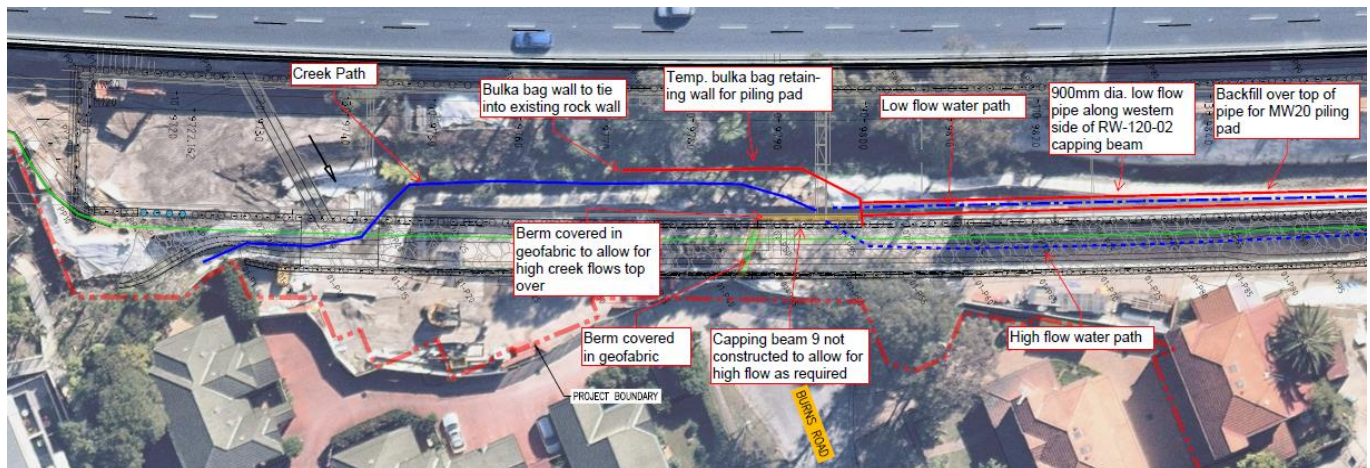
Figure 21: Environmental controls and work method for realignment of Cockle Creek behind retaining wall 2
