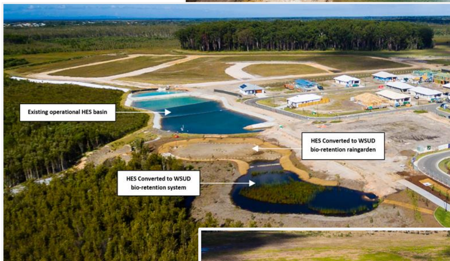
Figure 4.1.5 (left) - Aerial photo showing H5 HES basin water quality in background, and converted H4 HES to a wetland bio-retention system in foreground
