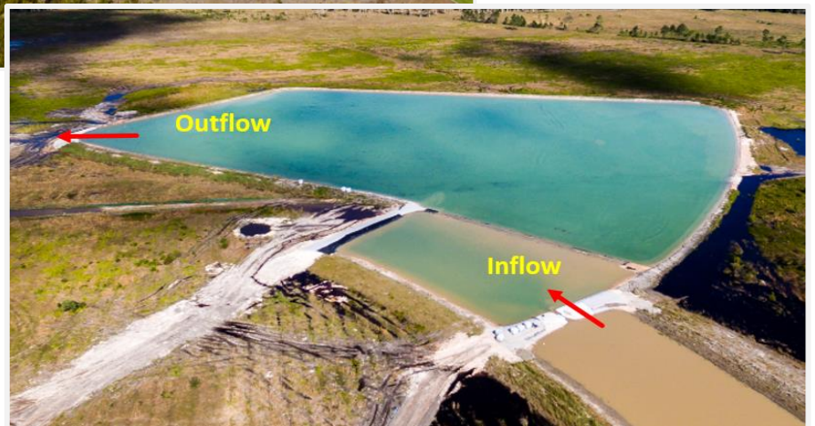
Figure 4.1.5 (left) - Aerial photo showing H5 HES basin water quality in background, and converted H4 HES to a wetland bio-retention system in foreground
