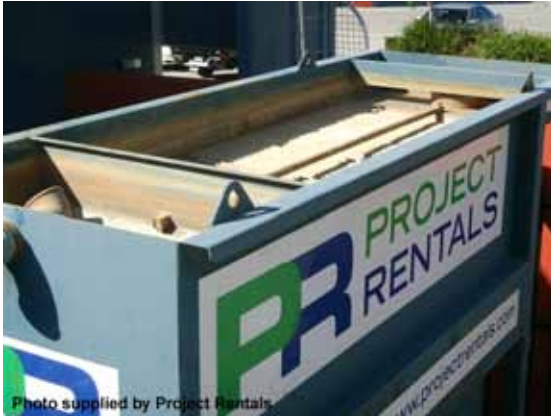
Lamella settling tank
