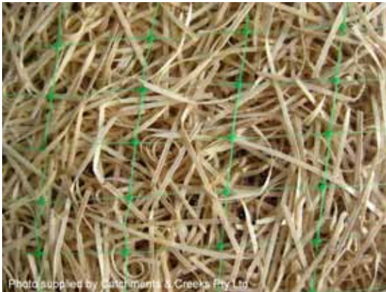
Temporary erosion control mat
