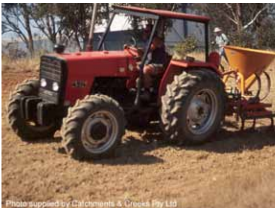
Scarifying the soil surface
