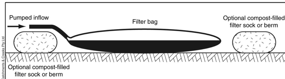
**Figure 4 – Placement of filter bag within a compost-filled filter sock enclosure**
