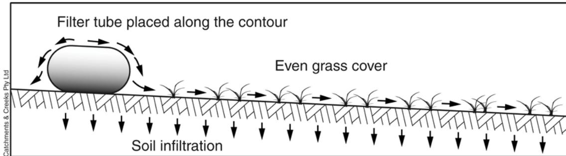
**Figure 1 – Ideal placement of filter bag or filter tube up-slope of a grassed filter bed**
