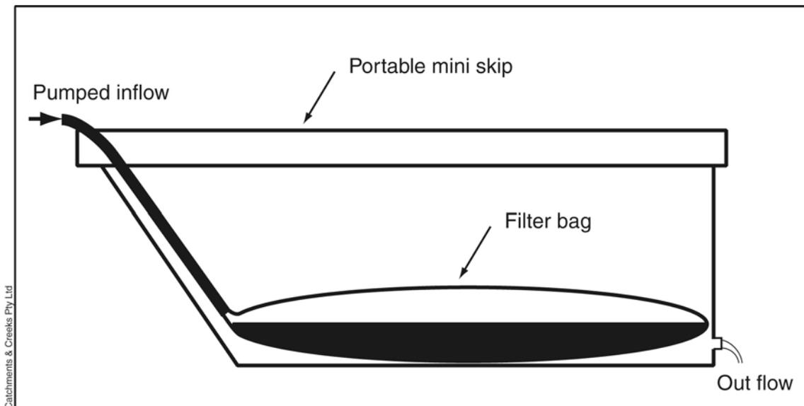
**Figure 2 – Placement of filter bag within a free-draining mini-skip**
