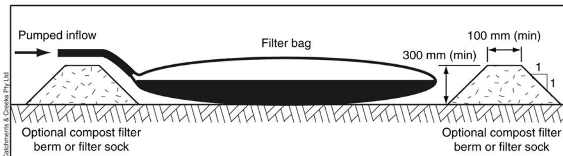
**Figure 3 – Placement of filter bag within a compost-filled filter berm enclosure**
