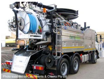
Photo 15 - Mobile treatment unit
