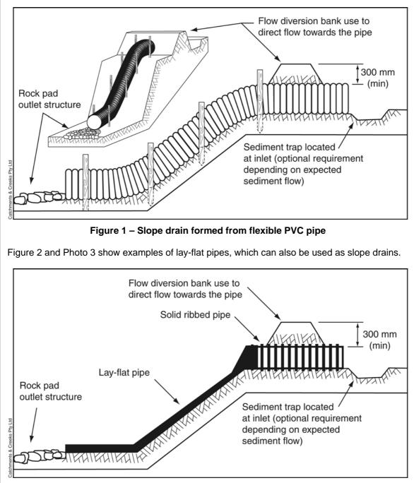
Figure 2 – Slope drain formed from lay-flat pipe
