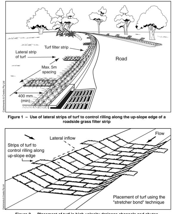
Figure 2 – Placement of turf in high-velocity drainage channels and chutes
