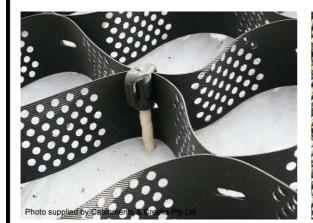
Photo 1 – Expandable, perforated sidewall, cellular confinement system
