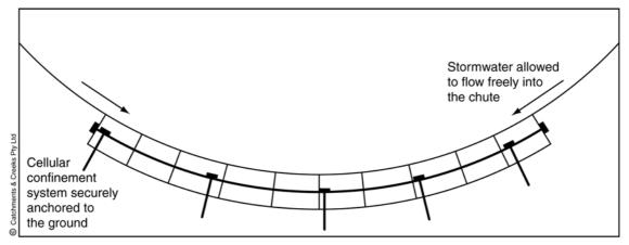
Figure 1 - Placement of cellular confinement system within a chute with concave profile
