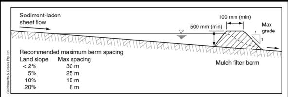
Figure 1 – Placement of mulch filter berms
