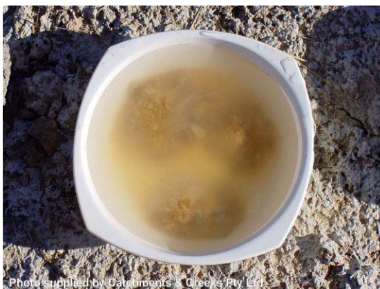
Photo 9 – Typical response of a dispersive or highly dispersive soil
