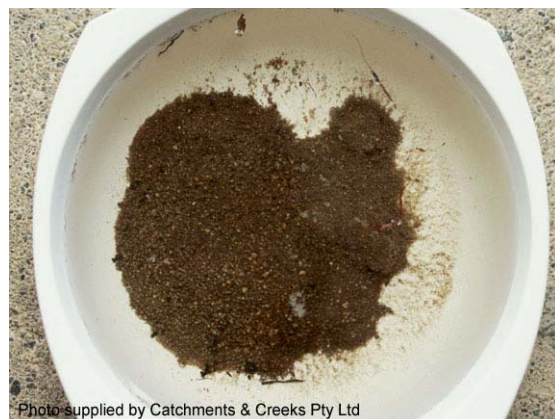
Photo 10 – Typical response of a slaking soil
