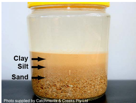
Photo 3 – Separate layers of clay, silt and sand visible in settled sample
