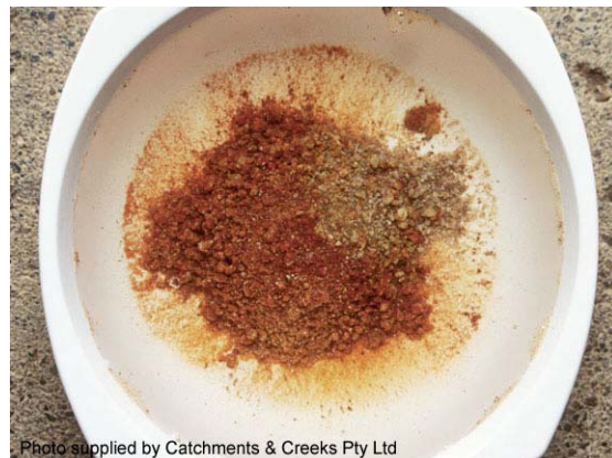
Photo 8 – Typical response of a slightly dispersive soil
