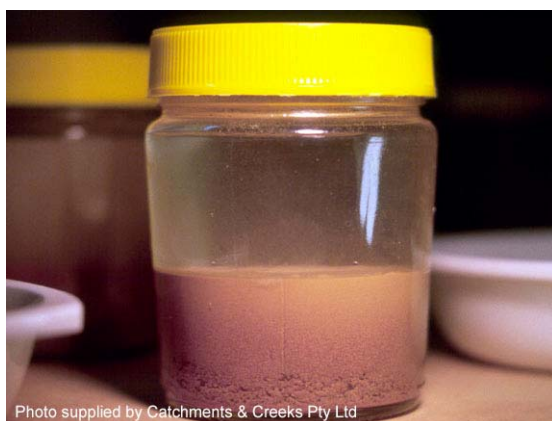
Photo 5 – Good settlement indicates soil is unlikely dispersive
