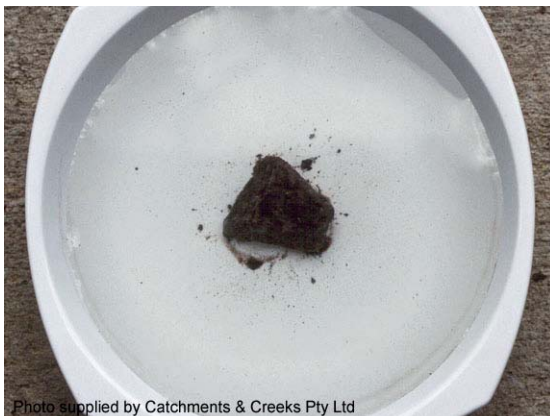
Photo 7 – Typical response of a non slaking, non dispersive soil
