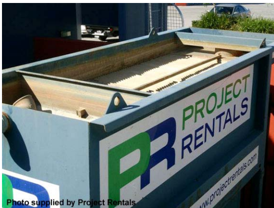
Photo 1 – Lamella settling tank
