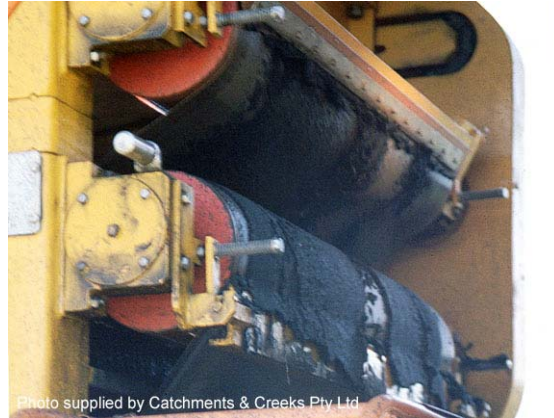
Photo 4 – De-watered sludge output from the de-watering of a sludge lagoon within a wastewater treatment plant
