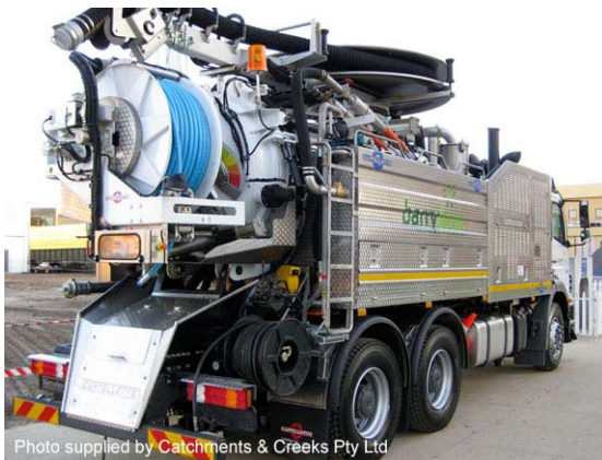
Photo 1 – Truck-mounted vacuum unit
