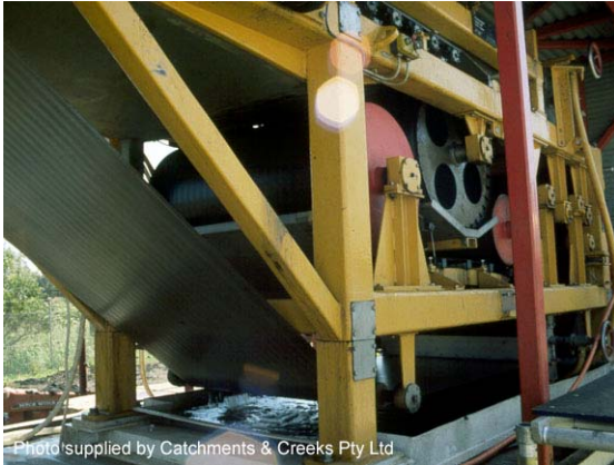
Photo 3 – Belt-press unit in operation
